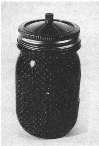
Fig. 1. Cell assembly for migration studies of plasticizers from PVC film into olive oil.
